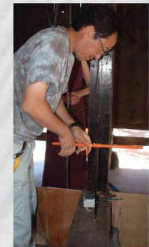
Architect FURIHATA learning wood sampling drilling, using a manual auger.
