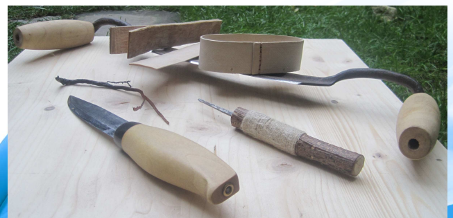
Used tools and materials: Draw knife, knife, awl, ash latewood bands, spruce roots
